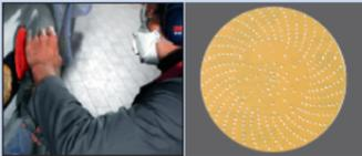
Spachtelschliff<br>Ponçage du mastic                                                    | P240 - P320      |                                   | 3M 236U Hookit Discs<br>3M 236U Hookit Discs                                                                                         |                                                                                                                                    |
